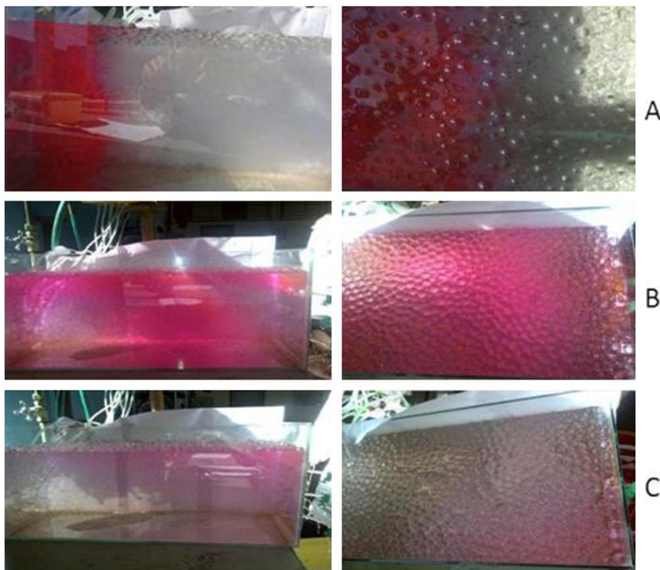
Figure 12. Photographs showing the flow patterns of tracer through the laboratory apparatus.
